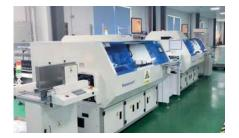
1. Universal Auto Insert Machine: Components automatically inserted to PCB, accurate and efficient.
